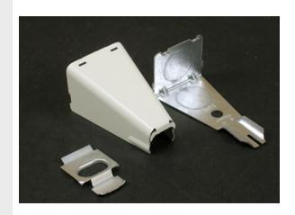
Connects raceway, without offsetting, to any surface-mounted 3 1/4" or 4" [83mm or 102mm] outlet box with 1/2" trade size conduit KOs. Base has two 1/2" trade size KOs, one on end and one on bottom. Included spring steel bushing eliminates need for conduit nipple and HICknut for end connection to box. When used with 700 Series Raceway, break off cover extension.
