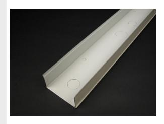
.040" [1.0mm] steel. Packed in ten 10' [3m] lengths, 100' [31m] per carton. Base sections have predrilled 1/2" and 3/4" trade size entrance KOs and 9/32" [7.1mm] dia. mounting screw KOs on approx. 9 3/8" [238mm] centers.
