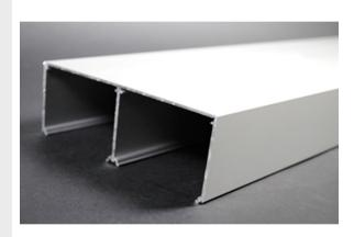
6063-T5 extruded aluminum, satin anodized finish, .078" [1.98mm] wall thickness. Bse has integral divider for seperation of service. Packed 40' [12m] per carton.
