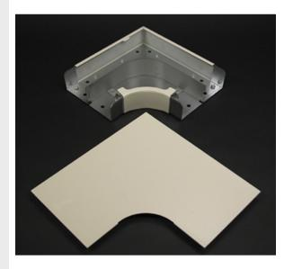
Full capacity 90 degree flat corner used in divided or undivided applications. Provides 2" [51mm] bend radius control for UTP, STP and fiber optic installations. Ideal for new installation when the cable is lay-in or pull-through.
