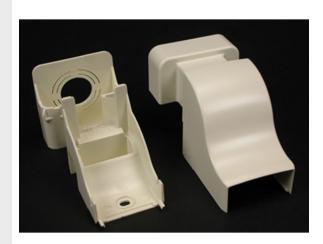
For dropping cables from ceiling into the raceway. Has 1/2" and 3/4" concentric trade size KOs. Includes PN153R Reducer Adapter for use with PN03 Series Raceway.
