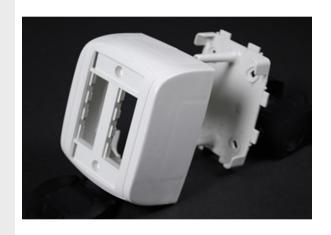
Surface mount box for use with Eclipse Raceway or standalone application. Has two 1/2" trade size KOs. Accepts four front-loaded downward facing Ortronics TracJack inserts.
