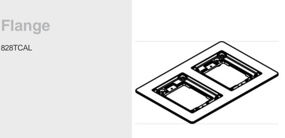
Two-gang brushed aluminum combination carpet and tile flange, 5.940" x 9.045" [150.9mm x 229.7mm]. Accepts Ortronics MAB6TJ TracJack and MAB3S2 Series II, and Wiremold CM Series Open System adapters, sold separately. NOTE: Brushed aluminum flanges come with beveled edges. Brass cover plates can only be used with brass flanges. Brushed aluminum flanges come with beveled edges.
