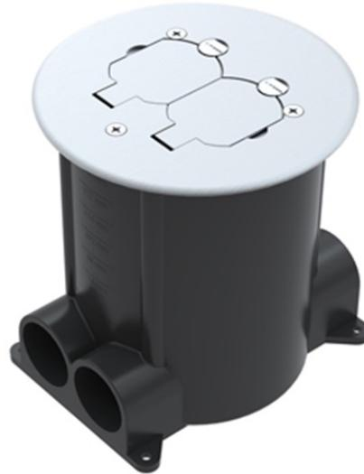
Supplied with reusable concrete cap, adapter ring, conduit reducers, and conduit hub plugs. Available for both single and dual service. Graduated cubic inch markings inside the box indicate volume capacity at any depth. Box has parallel conduit hubs eliminating the need for 90° sweeps in installation. One-piece reduction from 1" to 1/2" [25mm to 12.7mm] conduit. Reducers and plugs located on a mounting bar for easier selection. For concrete pours of 2 1/4" to 6" [57mm to 152mm].
