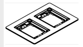
Two-gang brass combination carpet and tile flange, 6.080" x 9.185" [154.4mm x 233.3mm]. Accepts Ortronics MAB6TJ TracJack and MAB3S2 Series II, and Wiremold CM Series Open System adapters, sold separately. NOTE: Brass cover plates can only be used with brass flanges. Brushed aluminum flanges come with beveled edges.
