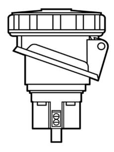
2 Pole, 3 wire, Pin and Sleeve Receptacle. 30 amp, 250 volt.
