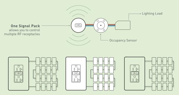
Control multiple dual- and half-controlled receptacles on the same circuit with feed-thru capability of the RF receptacle.
