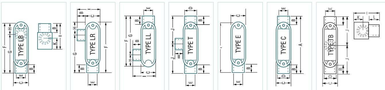
\* All access fittings are CSA certified and all access fittings except Type TB are UL listed for wet locations. Supplied with threaded brass inserts, combination brass head screws and PVC gasketing.
