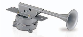
Model 52 resonating horn is ideal for penetrating high ambient noise levels. Being electrically-activated, the Model 52 does not require an expensive air compressor for operation. It is able to withstand the shocks, vibrations, dust and atmospheric conditions encountered in off-road use.
