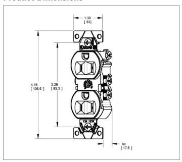
Figure 1. TR270 Line Art with Dimensions
