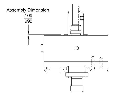
It should measure between .096 and .106 from the top of the block to the top of the bearing to obtain the proper spacing required for the location of the motor mounting plate.
