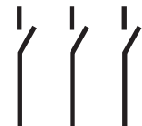
No Fuse, Two-pole, 240 Volts AC; 250 Volts DC (30-100 amps only); Three-pole, 240 Volts AC or Two-pole with Switching Neutral
