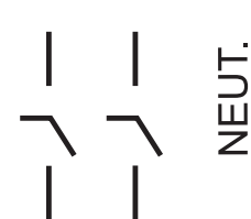
Three-wire SN, 120/240 Volts AC, No Fuse
