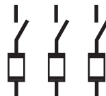
Fusible, Three-pole, 240 Volts AC and Three-pole, 480, 480Y/277 and 600 Volts AC-250 Volts DC, Fusible
