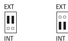
Figure 82: Connecting the external supply voltage with jumpers
