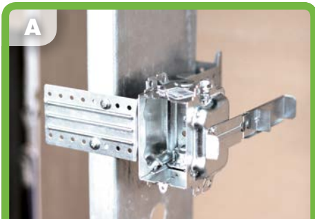
A Bend the mounting bracket to the right stud size using built-in guides. Install on either side of the stud.
