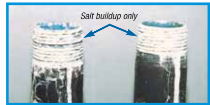
Examples of Hot-Dip Galvanized Threads after 42-day salt-fog test
