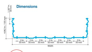
The 1/4 in. extension on the longtitudinal wires of QuikLok® tray profiles ensures that tray splices are strong and secure.
