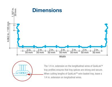
Note: To ensure electrical continuity, the Blackburn<sup>®</sup> **GPT-2** grounding connnector (see p. C30) and ground wire **MUST** be used in all QuikLok<sup>™</sup> Series tray applications.
