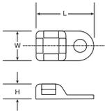
Four-way screw mounts for cable ties up to 50-lb. (222 N) tensile strength!
