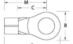
These non-insulated ring terminals are made of electrolytic copper for high conductivity. They can be installed with crimping tools having a single indentor or double indentor (recommended for solid
