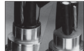
4. Pot cable (using liquid or putty)
