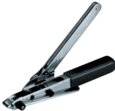
WTJ020 Lightweight pocket-sized tool to install 1/4" and 3/8" wide Free-End Clamps. This tool also applies tension and has a built-in cutter.
