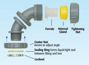
Arlington's no-spin ferrule allows the Zero to 90 connector to be secured to the conduit while fully assembled. To install, simply loosen the tightening nut and screw onto conduit. A positive liquid-tight seal is formed by the pressure sensitive internal gland as the nut is tightened. The sealing ring assures a liquid-tight seal between the fitting and box.
