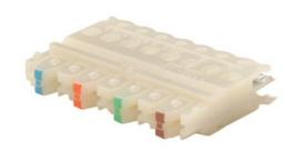
110C4s are four-pair, color-coded connecting blocks (clips) that are used to terminate 22- 26 AWG solid conductors onto 110 wiring blocks.
