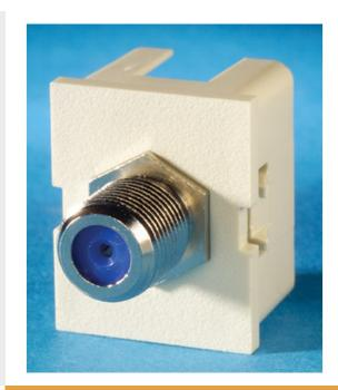
TracJack Module provides a single F-connector coupler F/F with under .2dB of insertion loss at 2GHz (1/3 the loss of standard models). TracJack is a versatile single jack solution in a front-load footprint which allows a choice of up to six jacks/connectors to fit in a single gang plate
