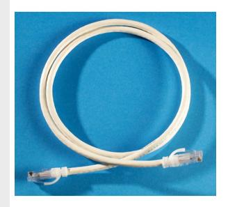
Clarity 6 Modular Patch Cord, white, 3', Category 6, four-pair UTP stranded 24 AWG PVC/CM, center tuned with Clarity 6 connecting hardware for optimum Category 6 installed performance using Paralign 2 pair-positioning technology
