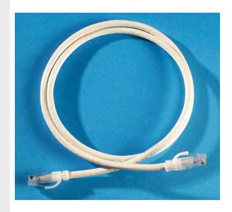
Clarity 6 Modular Patch Cord, white, 7', Category 6, four-pair UTP stranded 24 AWG PVC/CM, center tuned with Clarity 6 connecting hardware for optimum Category 6 installed performance using Ortronics Paralign 2 pair-positioning technology
