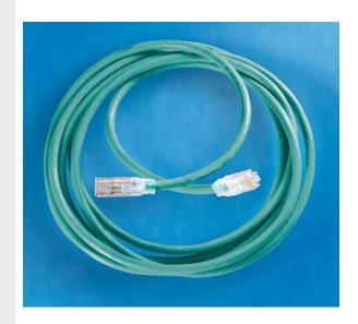
Clarity 5E Premium Category 5e Modular Patch Cord, blue, 3', four-pair UTP stranded 24 AWG PVC/CM, center tuned with Clarity 5E connecting hardware for optimum Category 5e installed performance using Ortronics Paralign 2 pair-positioning technology.
