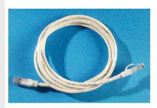
Clarity 5E Premium Category 5e Modular Patch Cord, white, 5', Category 5e, four-pair UTP stranded 24 AWG PVC/CM, center tuned with Clarity 5E connecting hardware for optimum Category 5e installed performance using Ortronics Paralign 2 pair-positioning technology
