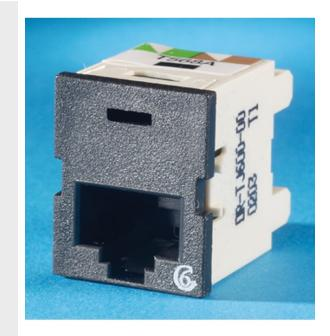
Clarity 6 TracJack, ETL verified to TIA Category 6 component specification. Frontloading and front removable. New universal T568A/B wiring label and tapered wiring towers simplify termination. Center tuned to Clarity 6 patch cords for optimum performance
