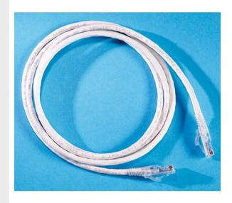
TechChoice modular patch cords are available in your choice of six lengths and seven colors. Each cable is pre-tested for component performance. This modular patch cord is Cat 5e, four-pair, AWG stranded, PVC, 7' long, white, sold in packages of 10.
