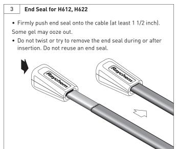
Note: The end seal is designed to be installed only once; it cannot be removed from the heating cable once installed. Do not use until ready for final installation.
