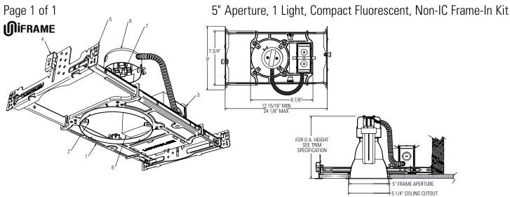
Complete Fixture consists of Frame-In Kit and Reflector Trim. Select each separately.
