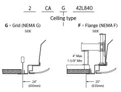
(NEMA Type G) Lay-in acoustical ceilings using exposed grid suspension, with tees for luminaires on 24" x 48" spacing. (NEMA Type F) Flange for acoustical ceilings using concealed mechanical suspension. Swing-jack mounting brackets: adjustment 4" max.and 1-5/8" min. Refer to sheet 801-CL for cut-out information.
