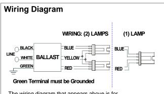
The wiring diagram that appears above is for the lamp type denoted by the asterisk (\*)
