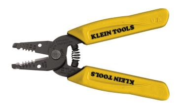
Complete electrical wiring tasks quicker by stripping 2 wires at a time with the Klein Tools 6-1/4-Inch Dual-Wire Stripper/Cutter. This tool is designed for use with 10-14 AWG solid wire. Its precision-ground stripping holes cleanly cut wire and aid in easy removal of insulation.
