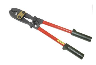
Use this crimping tool to crimp 6 - 4/0 AWG lugs and terminals. High-leverage handles and compound-action mechanism offer superior mechanical advantage. Ultra-comfortable hand grips for easy use and minimal fatigue. Adjustment screw allows user to control crimp depth.
