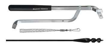
Klein's Flex Bit kit includes everything you need for drilling and pulling wire and cable. The flexible drill bit makes 9/16-Inch (14 mm) holes in wood. The folding placement tool helps guide the bit as you drill. The pulling grip attaches to the flexible drill bit after the hole has been made to pull wire and cable through.
