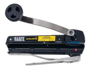
The Klein Tools BX and Armored Cable Cutter is simple to use. It easily cuts 3/8-Inch flexible conduit and #10, 12, and 14 armored cables with a couple of turns of the handle. Extra blades can be stored in the handle for convenience.
