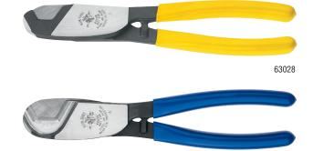
Cat. No Handle Color **Cutting Capacity** Handle Finish **Overall Length** Weight 63028 3/4" (19.1 mm) Yellow Plastic-Dipped 8.25" (209.6 mm) 0.80 lb (0.36 kg) 63030 Blue Plastic-Dipped 8.25" (209.6 mm) 0.83 lb (0.38 kg) 1" (25.4 mm)
