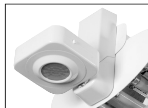
• Self contained line voltage sensor. Specifically designed to mount via the 7/8" KO provided on either end of the Trilyte luminaire. (Field Installed). Cat number MD360
