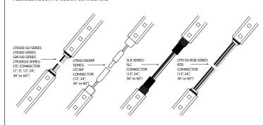
NOTE: Channels may not accommodate all ribbon to ribbon and ribbon to power supply connections. Please locate connections outside of channel interior.
