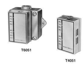
THE T4051, T6051, AND T6052 ARE HEAVY-DUTY, LINE VOLTAGE THERMOSTATS USED TO CONTROL FAN COILS, FANS, MOTOR STARTERS, VALVES, CONTACTORS, AND CIRCULATOR MOTORS IN HEATING AND/OR COOLING SYSTEMS.
