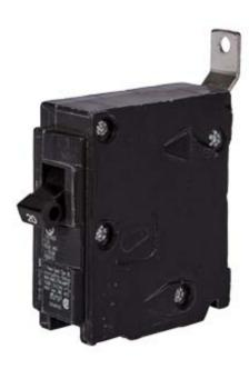
Siemens Low Voltage Molded Case Circuit Breakers Panelboard Mounting 240V Circuit Breakers - Type BL, 1-Pole, 120VAC are Circuit Protection Molded Case Circuit Breakers. Type: BLH Application: Electrical Distribution Standard: UL 489 Voltage Rating: 120V Amperage Rating: 15A Trip Range: Thermal Magnetic Interrupt Rating: 22 AIC Number Of Poles: 1P
