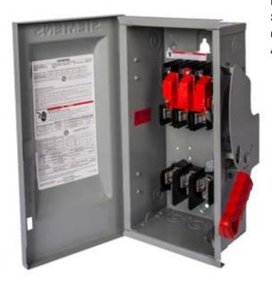
Siemens Low Voltage Circuit Protection Heavy Duty Safety Switches. Type: ENCLOSED, SAFETY SWITCH Std: CSA V. Rating: 240V A. Rating: 100A Wattage: 4W No. Of Poles: 3P F. Rating: 60Hz Action: SINGLE THROW Material: 304SS Enclosure: TYPE 3R. 2-3 point mounting holes. O. Cycles: 10000 O. Temperature: (-20F-120F) AMBIENT TEMPERATURE Environmental Conditions: OUTDOOR
