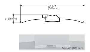
Controls sensor integrated into one lens retainer.
