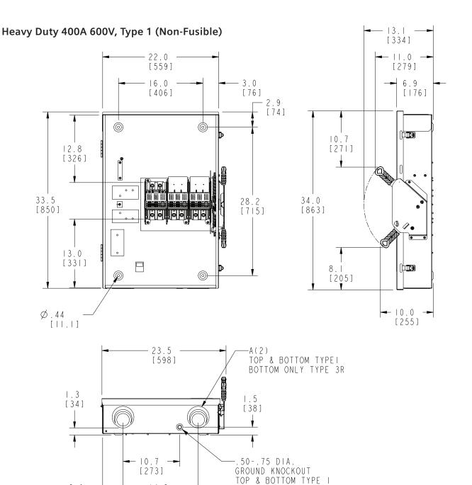
Dimensions shown in inches and millimeters [ ]. Dimensions shown accurate to  $\pm$  1/8 inch.
